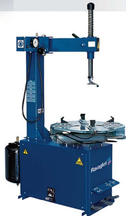
The pedal assembly can be removed as an integral unit allowing easy servicing.
