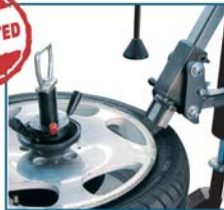
The tool enters between bead and rim
