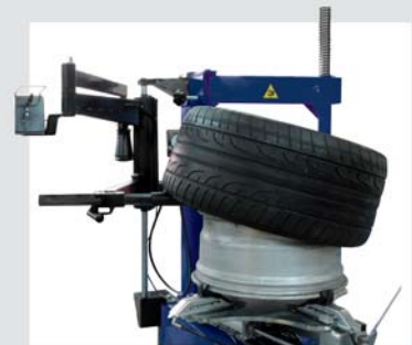
DEMOUNTING (lower bead)
