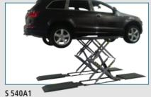
Kit with additional run up ramps for low ground clearances vehicles
