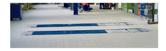
Hydraulic levelling system by means of a patented synchronisation device assures constantly level lifting platforms regardless of weight distribution.
